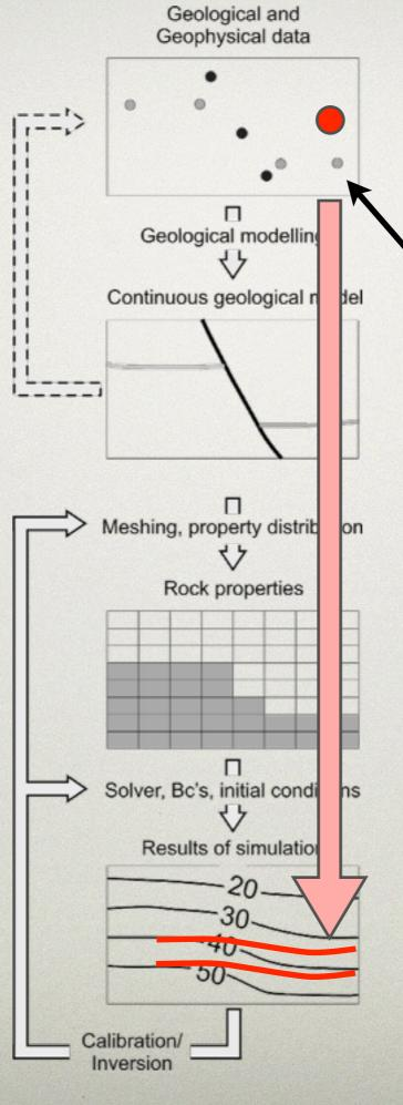
Now possible: change position of geological data point, automatically update effect on simulated flow fields Developed methods to combine implicit modelling and input file generation with PySHEMAT and PyTOUGH (both open source, available on github.com)
