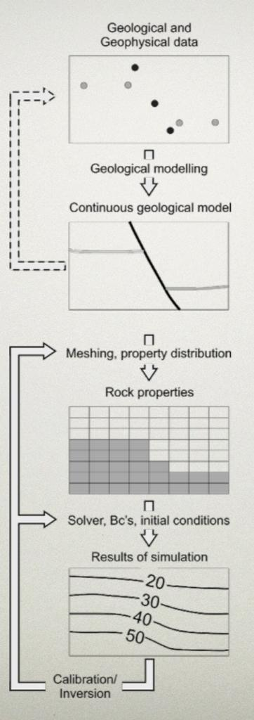
Developed methods to combine implicit modelling and input file generation with PySHEMAT and PyTOUGH (both open source, available on github.com)
