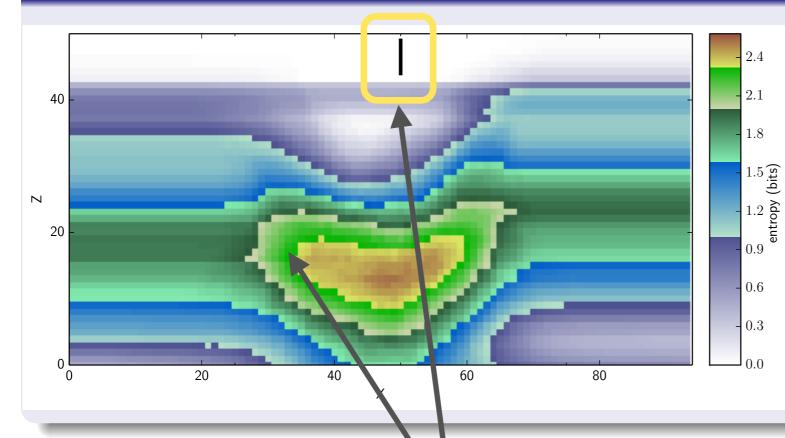
Conditional entropy of each cell given information at subsequent locations along a line ("drillhole"): uncertainty in the model is reduced with new knowledge.
