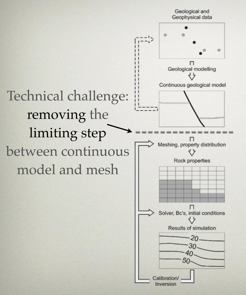
**Developed** methods to combine implicit modelling and input file generation with PySHEMAT and PyTOUGH (both open source, available on github.com)
