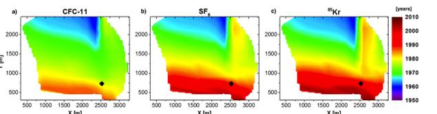
Map of the apparent ages obtained with the in-silico model in the contact zone of the Plœmeur site. Contour of the map is determined by taking the supplying limit of the pumping well. From left to right: CFC-11, SF<sub>6</sub> and <sup>85</sup>Kr apparent ages. The pumping well is identified by the black square.
