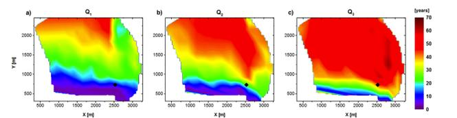
Map of the different renewal times (from left to right, times at which 25, 50 and 75% of the water is renewed corresponding to  $Q_1$ ,  $Q_2$ , &  $Q_3$ ) obtained with the in-silico model. The pumping well is identified by the black square.
